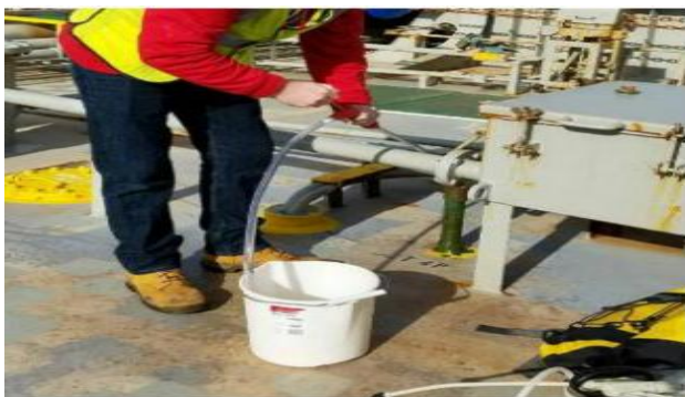
Figure 3: Taking a sample of a ship's ballast water tank.
