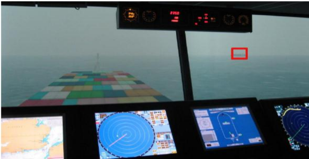
Figure 1, Highlighted target, using red box, is projected into the bridge window. Source: (Accseas, 2015)
