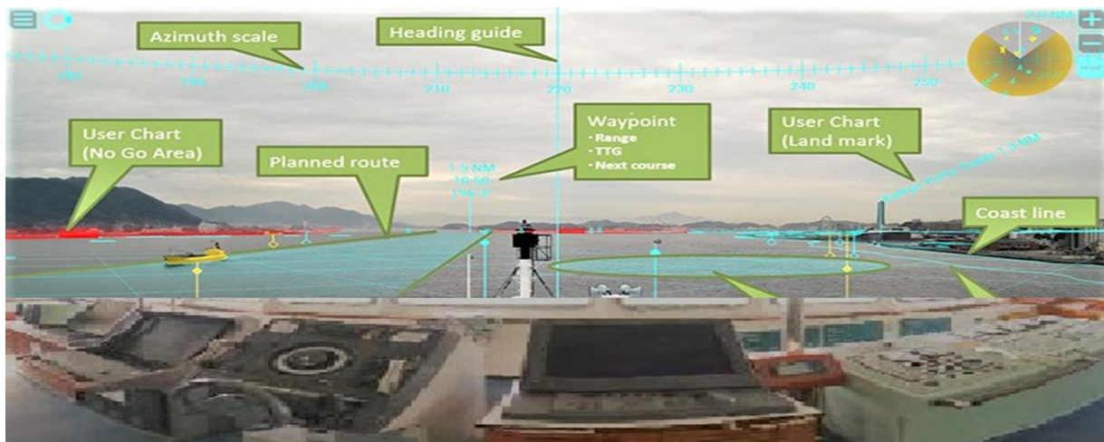
Figure (7) AR Navigation System onboard Aida4 ship.
