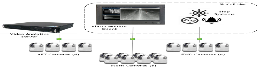
Figure 3: Infrared human motion detector System Diagram. (Pure tech, 2015)
