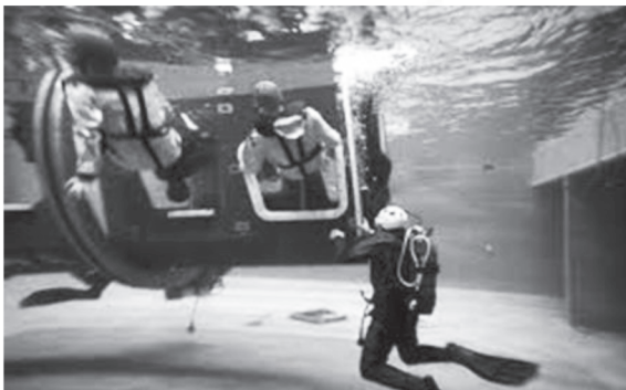
Figure (2): Helicopter Under Water Escape Training Simulator Source: MSI-AAST&MT. 2020a
