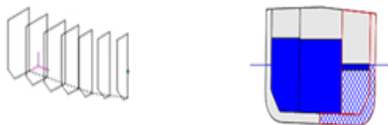
FIG 8 case 5 damage in 15 meter from bottom
