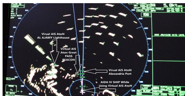
Figure (4): The ship Aida IV during the implementation of the practical experiment in the port of Alexandria.
