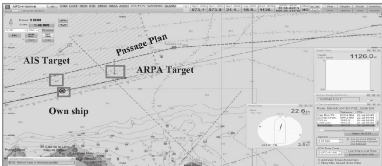
Figure 1: ECDIS interface integrated with ARPA & AIS Source: AASTMT ECDIS Simulator
